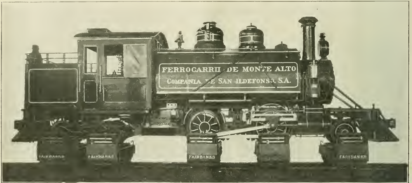
BALDWIN'S METHOD OF WEIGHING LOCOMOTIVES. NO GUESSING HOW MUCH WEIGHT IS ON EACH PAIR OF WHEELS.
